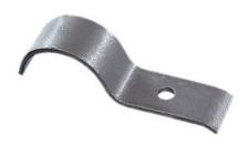
This fitting is used to attach profiled sheeting material to pipe. The fitting is supplied with the following hardware: one M6x50mm roofing bolt, one M6 square nut, and one M6 lock washer. BZP finish. Ø indicates diameter of bolt hole.
