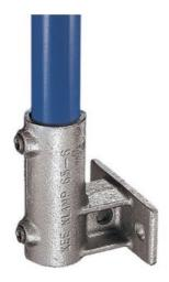
This fitting is designed for palm fixing guardrailing and balustrading to walls, parapets, steps and ramps. Only available in size 6. The upright cannot drop through the socket. Ø indicates diameter of fixing holes. Should an upright be required to pass through the fitting, the base can be bored out to order.
