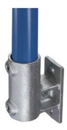
This fitting is designed for fixing guardrailing and balustrading to walls, parapets, steps and ramps. The upright cannot drop through the socket. Access to the top fixing hole is restricted by the position of the flange to the barrel. When selecting a hexagon head bolt or similar bolt fixing, the maximum length of the bolt including the head must not exceed 1". Should an upright be required to pass through the fitting, the base can be bored out to order. Ø indicates diameter of fixing holes.
