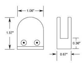
816FM glass grips are made of 304 grade stainless steel, are available in polished and satin (brushed) finishes, have a flat back for mounting on flat surfaces and come with a rubber insert set designed to hold  $\frac{1}{2}$ " thick panels.
