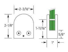
The 40-816F radius glass grip is made of 304 grade stainless steel, has a polished finish, a flat back for mounting on flat surfaces and comes with a rubber insert set designed to hold  $\frac{1}{4}$  -  $\frac{3}{8}$ " thick panels.
