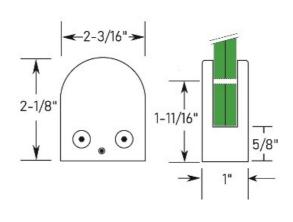
The 02-816F radius glass grip is made of brass, has a polished and clear coat (lacquer) finish, a flat back for mounting on flat surfaces and comes with a rubber insert set designed to hold  $\frac{1}{4}$  -  $\frac{3}{8}$ " thick panels.
