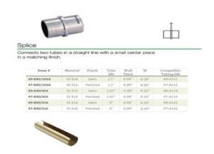
The 00-830/2 splice is an internal tube splice that is made of brass and fits entirely on the inside of a tube. It is designed to connect the ends of two tubes that are 2" round with a wall thickness of 0.05".
