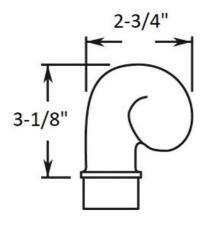
This decorative brass finial is made of brass and has a polished finish. It is to fit into tube with a 1-1/2" outside diameter and a 0.05" wall thickness.
