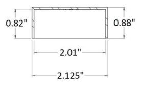
44-600W/2 is made of 304 grade stainless steel and has a satin (brushed) finish. It is designed to fit OVER a round tube or rod (wood included) that has a 2" outside diameter.
