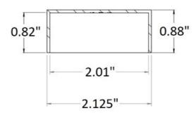
40-600W/2 is made of 304 grade stainless steel and has a polished finish. It is designed to fit OVER a round tube or rod (wood included) that has a 2" outside diameter.
