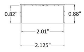
00-600W/2 is made of brass and has a polished finish. It is designed to fit OVER a round tube or rod (wood included) that has a 2" outside diameter.
