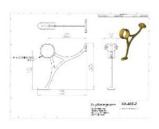
The 400 Combination Bar Footrail Bracket is available in sizes designed to hold 1-1/2" and 2" round tube and is available in brass and 304 grade stainless steel. Combination brackets are the most popular footrail brackets with one leg that mounts to the bar and the second leg that rests on the floor.
