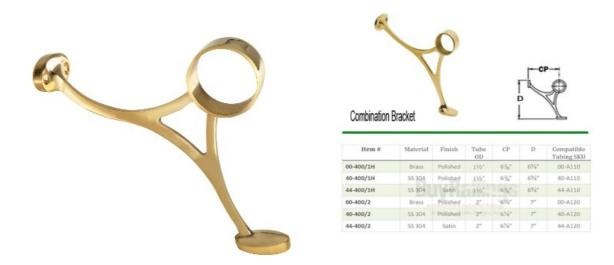
The 400 Combination Bar Footrail Bracket is available in sizes designed to hold 1-1/2" and 2" round tube and is available in brass and 304 grade stainless steel. Combination brackets are the most popular footrail brackets with one leg that mounts to the bar and the second leg that rests on the floor.
