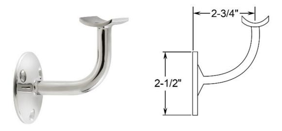
This wall mount handrail bracket is made of 304 grade stainless steel, has a polished finish and is designed to hold 2" outside diameter round tube. The back plate has three counter sunk holes that can be positioned for horizontal or angled handrail. Mount this bracket on a wall (recommended on a stud) or on a rectangular vertical post using the included hardware or alternate depending on the material the bracket is being mounted upon.
