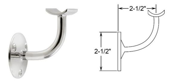
This wall mount handrail bracket is made of 304 grade stainless steel, has a polished finish and is designed to hold 1-1/2" outside diameter round tube. The back plate has three counter sunk holes that can be positioned for horizontal or angled handrail. Mount this bracket on a wall (recommended on a stud) or on a rectangular vertical post using the included hardware or alternate depending on the material the bracket is being mounted upon.
