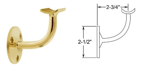
This Wall mount handrail bracket is made of brass, has a polished finish and is designed to hold 2" outside diameter round tube. The back plate has three counter sunk holes that can be positioned for horizontal or angled handrail. Mount this bracket on a wall (recommended on a stud) or on a rectangular vertical post using the included hardware or alternate depending on the material the bracket is being mounted upon.
