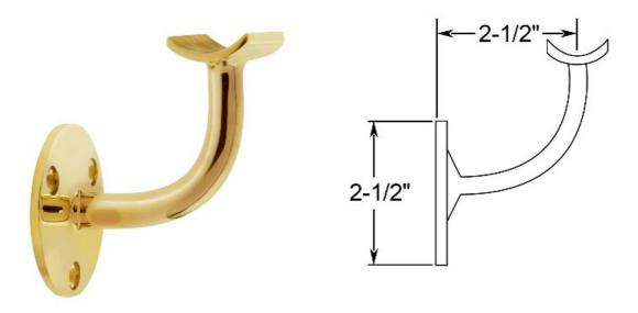
This wall mount handrail bracket is made of brass, has a polished finish and is designed to hold 1-1/2" outside diameter round tube. The back plate has three counter sunk holes that can be positioned for horizontal or angled handrail. Mount this bracket on a wall (recommended on a stud) or on a rectangular vertical post using the included hardware or alternate depending on the material the bracket is being mounted upon.
