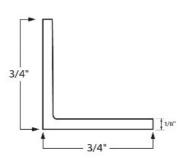
Our Brass Angles are made of 385 alloy brass and have two legs of equal length that form a 90 degree angle. Each angle is 12ft in length. Measurements in the item description list the leg lengths first followed by the leg thickness.
