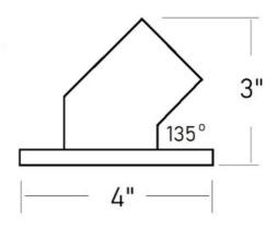
This 45 degree angle flange is an optimal solution to build angled sneeze guards or to terminate a tube from a 45 degree angle to a wall. 00-535/2 is made of polished brass and is for tube size 1-1/2" OD x 0.05" wall. The mounting flange has three counter sunk holes.
