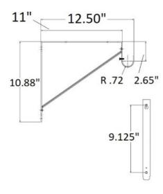
Our premium chrome finish closet brackets give dual support for both closet rods and shelving. Made from the highest quality metals and hand polished for a superior finish, they feature a set-screw that firmly locks and holds the closet rod into place.
